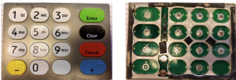
Fig. 9: Pin pad overlay used to collect PIN numbers
