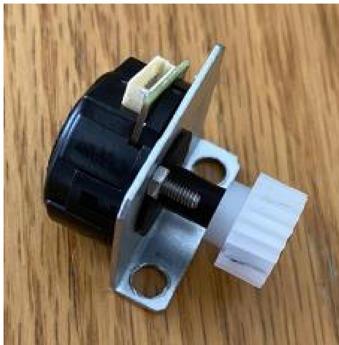
Fig. 23: 24 Inch Actuator 3D Printed Encoder Setup
