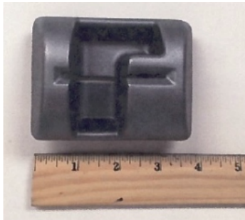
Fig. 5: Front of a typical overlay skimmer
