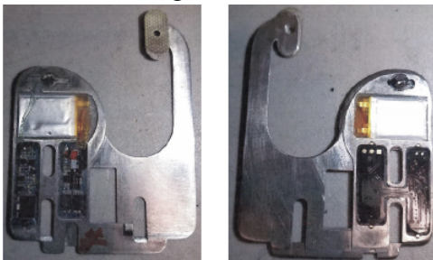
Fig. 7: Front and back of deep insert skimmer
